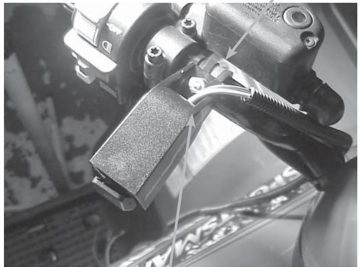
2. Mount Rocker Switch housing to Tube Clamp using #10 capscrew, locknut, flat washer, and shake-proof washer (items #14-3, #14-5, #14-8, and #14-9). Tighten securely.
